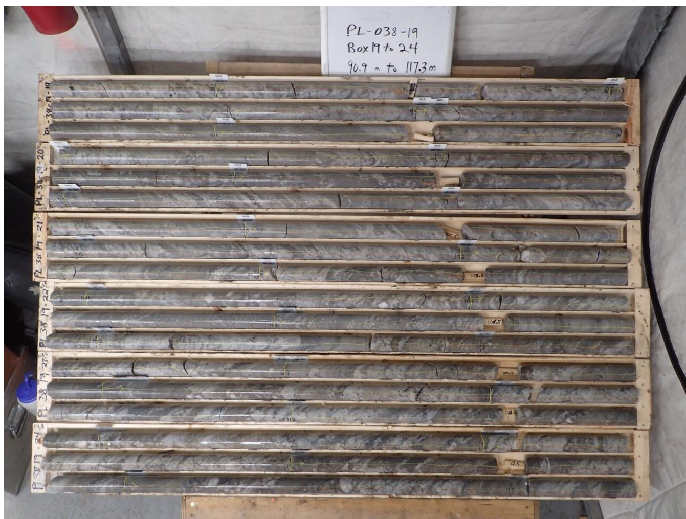
Figure 4: Spark pegmatite intersection hosting approximately 20% spodumene mineralization
