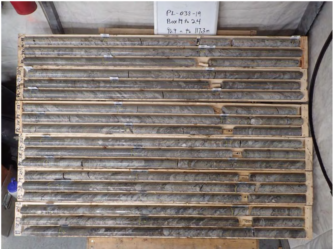
Figure 4: Spark pegmatite intersection hosting approx. 20% spodumene mineralization
