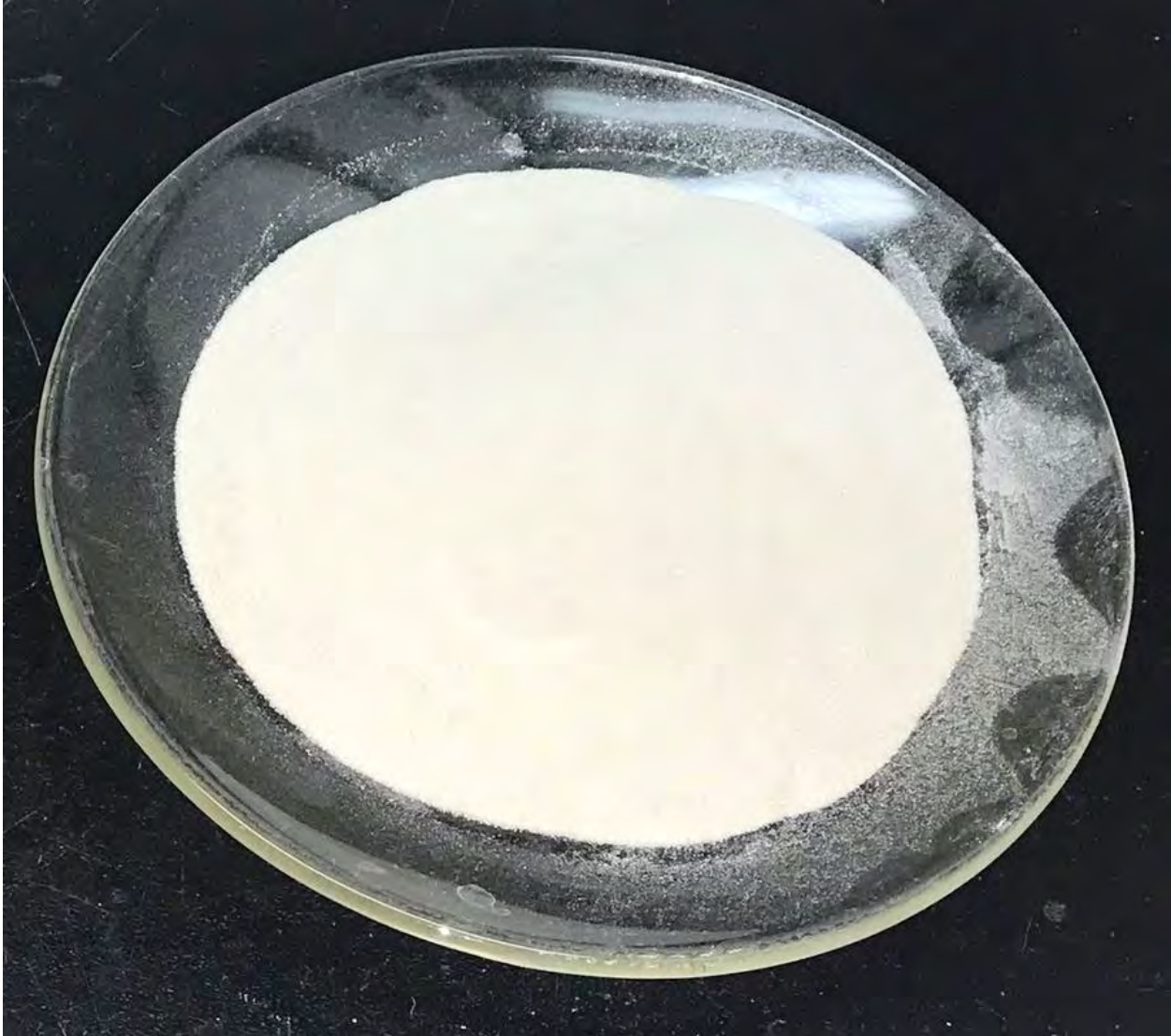
Figure 5: Frontier Technical Grade Spodumene sample containing 7.13% Lithium oxide and .15% iron oxide
