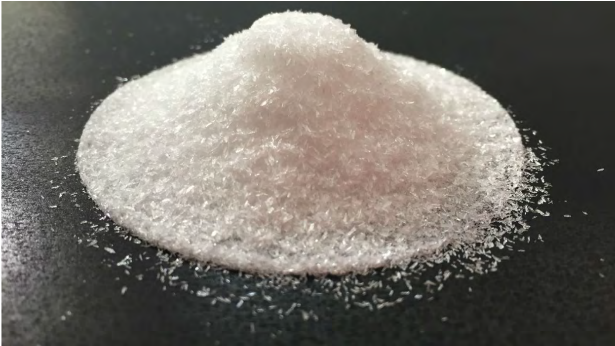
Figure 6: Sample of Lithium Hydroxide Monohydrate salt containing 35.6% lithium oxide
