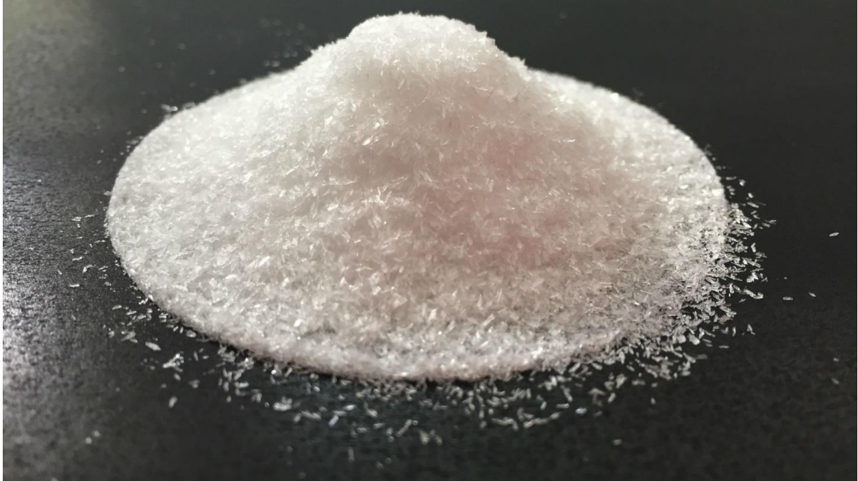
Figure 6: Sample of Lithium Hydroxide Monohydrate salt containing 35.6% lithium oxide
