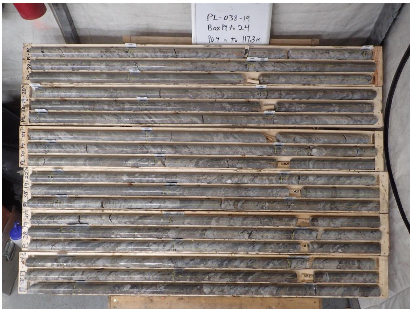
Figure 4: Spark pegmatite intersection hosting approx. 20% spodumene mineralization
