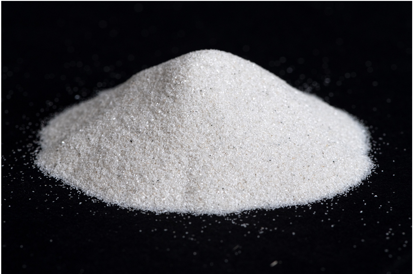
Figure 5: Frontier Technical Grade Spodumene sample containing 7.2% lithium oxide and .13% iron oxide
